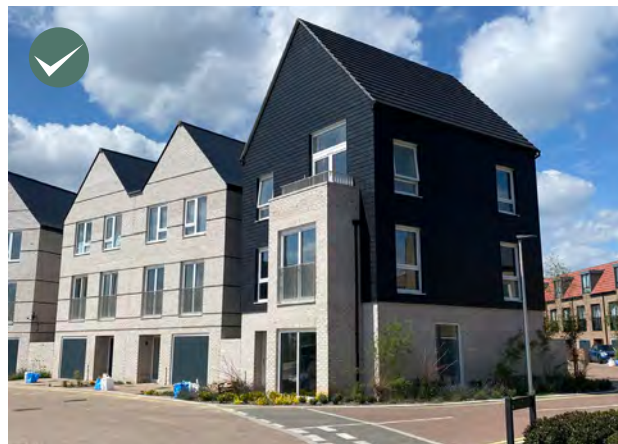
Marker building with architectural features and building ‘turning the corner’ with windows and doors onto both sides.
